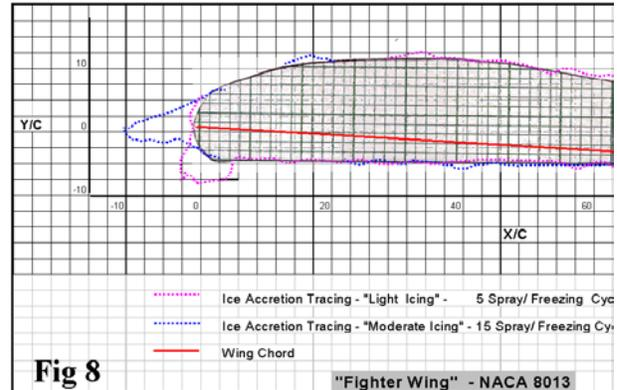
leading edge. For 'moderate icing', this structure grew significantly. Fig 9 shows a 63% decrease in lift at 20 deg AOA for 'moderate' ice vs. the 'clean' wing.
