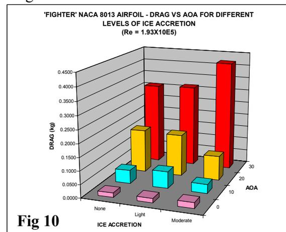
icing' there was less drag at 10deg and 20deg. AOA, (Fig 10) than the 'clean' airfoil. At 30deg. AOA the drag force doubled from 20deg. AOA. At 30deg AOA, the lift performance was greater than either the 'clean' or 'light icing' airfoil. The maximum L/D for all three icing conditions was 10 deg. AOA. L/D performance was approx. 50% less at 0 deg. AOA with 'moderate icing', than with either 'clean' or 'light icing'.
