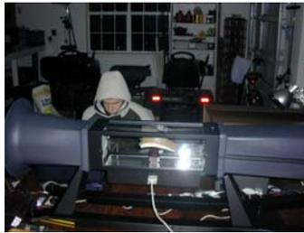
temperatures were near 0 deg C to prevent the ice from melting. The 'clean wings' were also tested to provide a baseline for data
