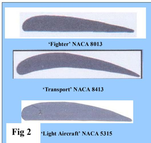
cardboard templates. I used the templates to cut the three airfoil shapes out of balsa wood, using a band saw, and then sanded the airfoils down into smooth wing shapes. Each of the three templates was compared to a wing form library that contains NACA designation numbers.
