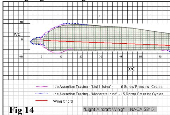
the airfoil. For the 'moderate' ice conditions, a large horn developed on the leading edge. For the 'Light Aircraft' airfoil, after passing 20kph, the lift performance of the 'moderate iced' airfoil started to drop and the drag
